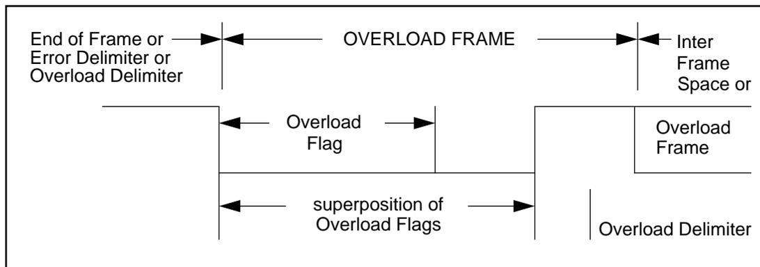
At most two OVERLOAD FRAMES may be generated to delay the next DATA or REMOTE FRAME.
