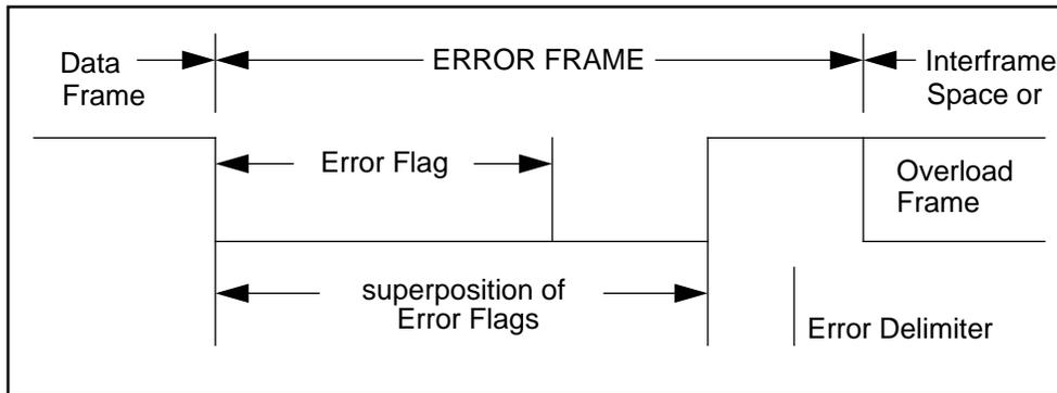
In order to terminate an ERROR FRAME correctly, an 'error passive' node may need the bus to be 'bus idle' for at least 3 bit times (if there is a local error at an 'error passive' receiver). Therefore the bus should not be loaded to 100%.
